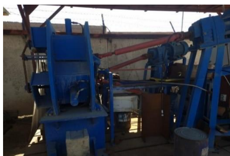
Figure 2 – The developed radial shear mill on the basis of KazNRTU named after K.Satpayev
