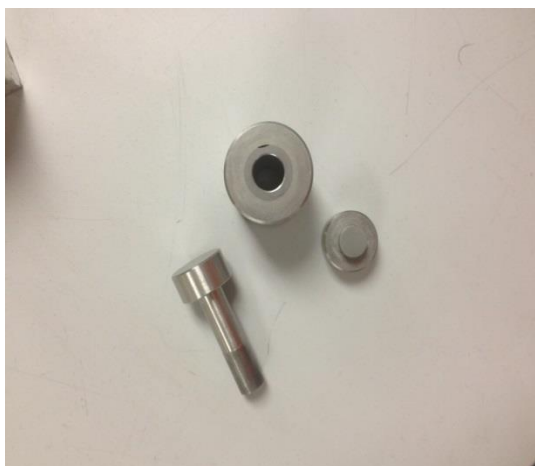
Figure 1 - Molding Dye Used for Pressing Silicon Carbide
